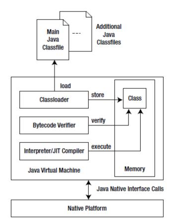
**Figure 1.2:** The JVM provides all of the necessary components for loading, verifying, and executing a classfile
