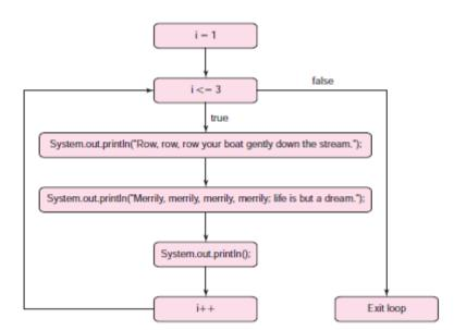
Figure 1.27 shows the program flow of this segment.
