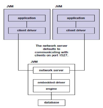
**Fig 1.4:** Multiple clients communicate with the same database engine through the network server.
