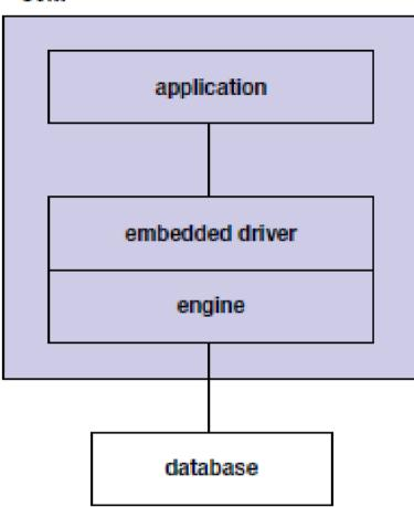
Figure 1.3: No separate processes are required to start up or shut down an embedded database engine.
