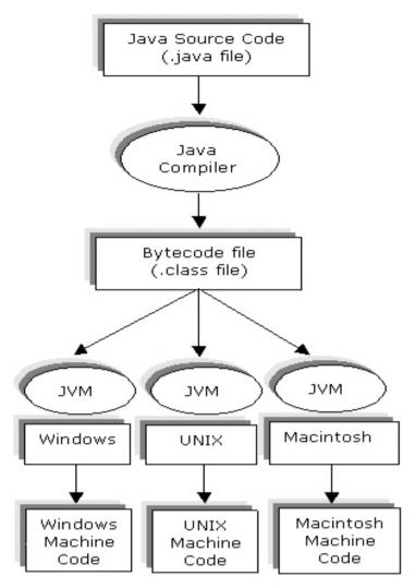
**Figure 1.1:** The Java compiler translates Java source code into Java object code consisting of bytecode and associated data
